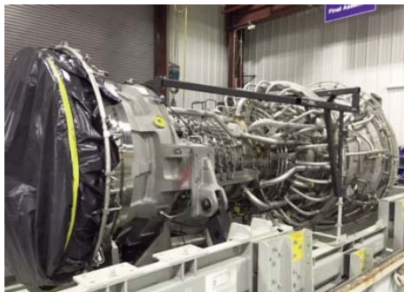
Turbines fired with natural gas can provide high horsepower for electrical generation when space is limited
